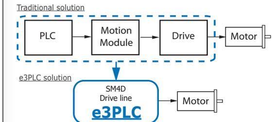
The e3PLC IDE allows the user to access all the I/O control functions and resources, provided by the drive, and to locally program its Motion Control Module, which can also be synchronized with other drives and events of the controlled process. Thanks to the advanced functionalities of the Power Motion Module, an integrated Real-time Process Module, applications can be easily created for special applications such as:
