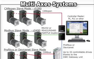
Drive control through commands by Master Controller. Suitable for multi axes systems (up to 127 drives). Built in Powerfull Motion Module functionality assures Perfect Synchronization among axes and reduces Master Controller
