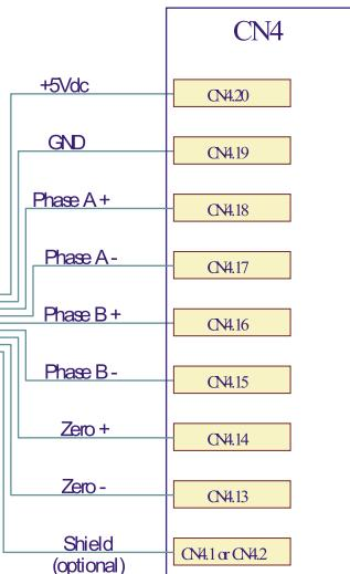
Single-Ended 5Vdc TTL/CMOS digital inputs
