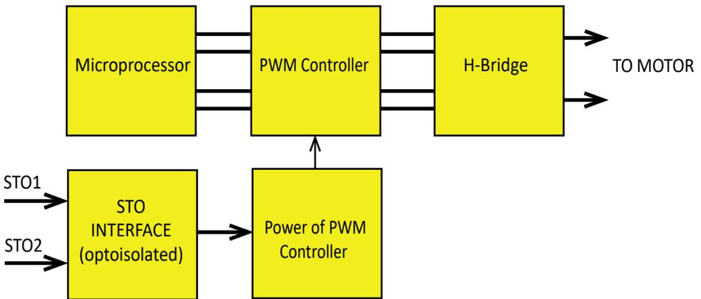
The drive has a safety feature that is designed to provide the Safe Torque Off (STO) function. Two input signals are provided which, when not connected, prevent the upper and lower devices in the PWM outputs from being operated by the digital control core. This provides a positive OFF capability that cannot be overridden by the control firmware, or associated hardware components.
