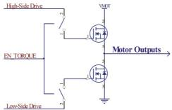
This is the enable signal for H-bridges that cannot be overidden by the control firmware:
