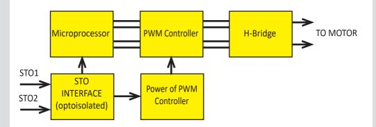
The drive has a safety feature that is designed to provide the Safe Torque Off (STO) function. Two input signals are provided which, when not connected, prevent the upper and lower devices in the PWM outputs from being operated by the digital control core. This provides a positive OFF capability that cannot be overridden by the control firmware, or associated hardware components.
