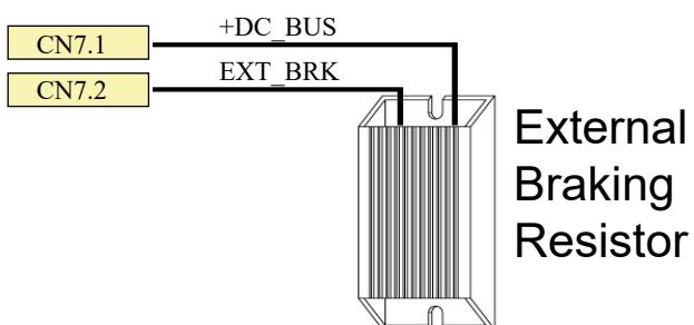
**External braking resistor must be placed more than 50mm from the drive on nonflammable and heat resistant surfaces. The metal case of the braking resistor can reach high temperatures. Take all necessary measures to avoid possible contacts in the final installation.**
