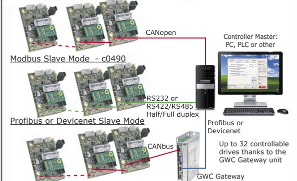
Drive control through commands by Master Controller. Suitable for multi axes systems (up to 127 drives). Built in Powerful Motion Module functionality assures Perfect Synchronization among axes and reduces Master Controller workload.
