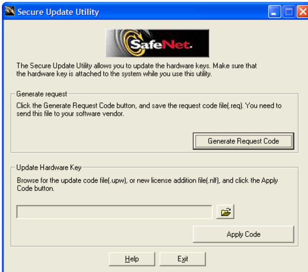
With the USB Hardware key inserted in the PC, press the 'Generate Request Code' and send the created .req file to EVER support/customer care. To update/upgrade your license, load the .upw/.nlf file sent by EVER pressing on
