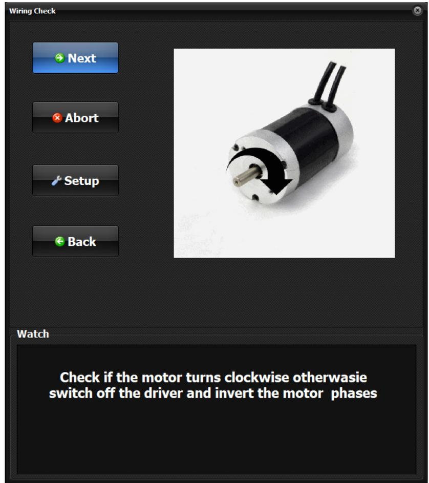
On the following page user tests if the set poles and gearbox are correct.
